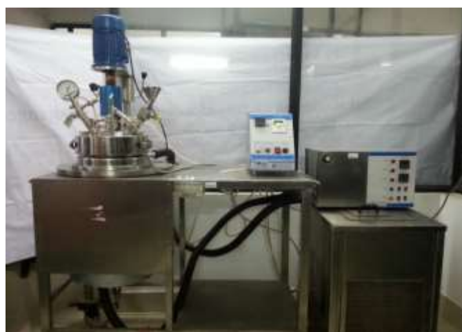
Fig: Image of the bioreactor developed for the Biodiesel production
